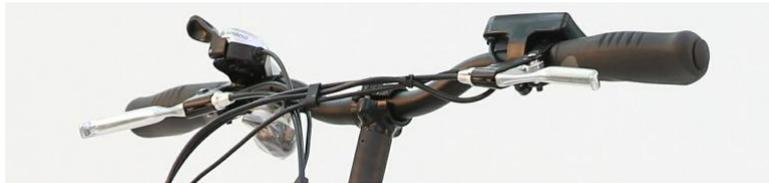
The left brake lever controls the front brake. The right brake lever controls the rear brake.
